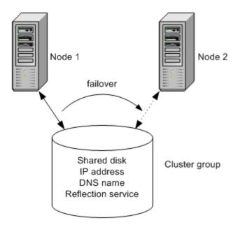
In the cluster above, if the Reflection for Secure IT service fails on Node 1, Node 2 acquires the shared resources and the Reflection for Secure IT service is started on the new node. At this point, Node 1 no longer has access to resources within the group. The Reflection for Secure IT server continues to run using the same configuration, so no change is apparent to clients establishing a new connection.
