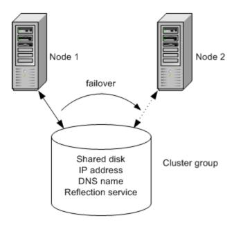
In the cluster above, if the Reflection for Secure IT service fails on Node 1, Node 2 acquires the shared resources and the Reflection for Secure IT service is started on the new node. At this point, Node 1 no longer has access to resources within the group. The Reflection for Secure IT server continues to run using the same configuration, so no change is apparent to clients establishing a new connection.
